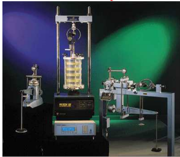
Triaxial equipment originally designed in Harvard university
