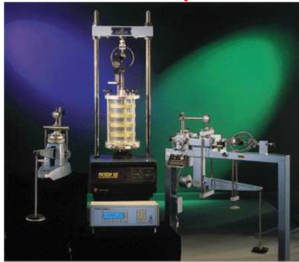
Triaxial equipment originally designed in Harvard university
